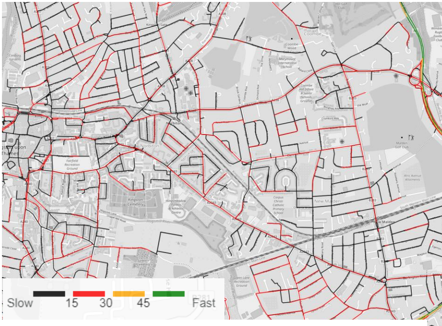
Highways Analyst map showing average speed in Kingston in the morning peak
